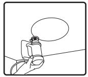
**3.** Use RotoZip or other tool to cut hole. Hole diameter: 5.6 in. (142 mm).
